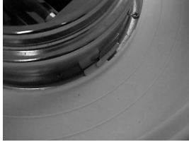
Figure C Metal tab on unit fitted with plastic tab on bowl to Lock and Unlock extractor head
